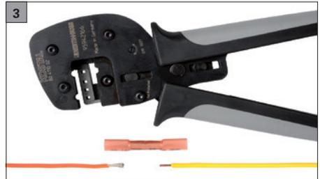
A crimp or shrink connector for example can be used for connection. These connectors are included in the scope of delivery.
